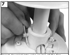
Insert downrod into yoke on top of the Fan Body. Align the hole in the Downrod with the hole in the Yoke. Insert the Pin through the Yoke and Downrod until the point appears on the other side. Install the keeper to pin.
